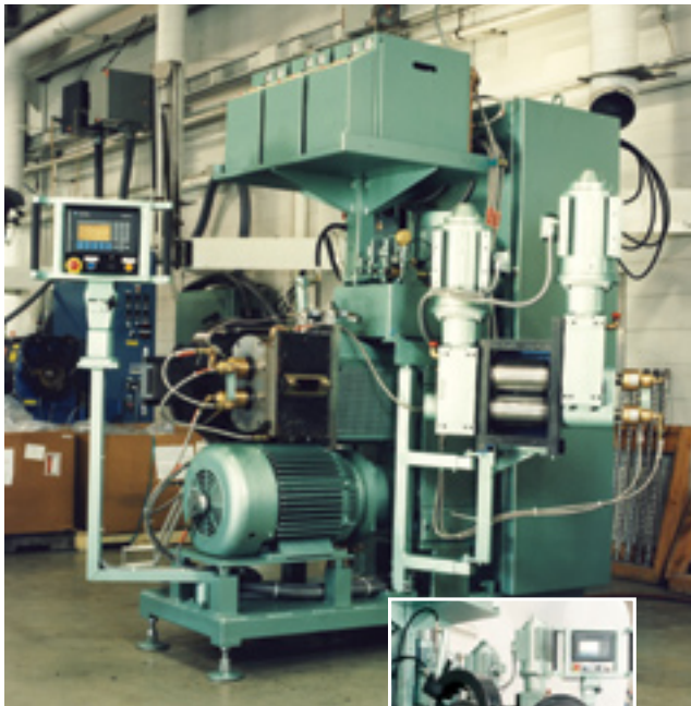
Swing-out two-roll feeder allows single-feed strip operation.
