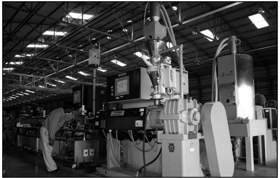
Polyhose has one of the most modern manufacturing facilities in Southeast Asia. Pictured is the company's existing Davis-Standard extrusion line.
