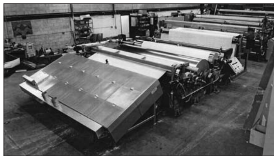
InterWrap's tandem extrusion coating line will be one of the fastest in India with line speeds of 700 feet per minute (213 meters per minute).
