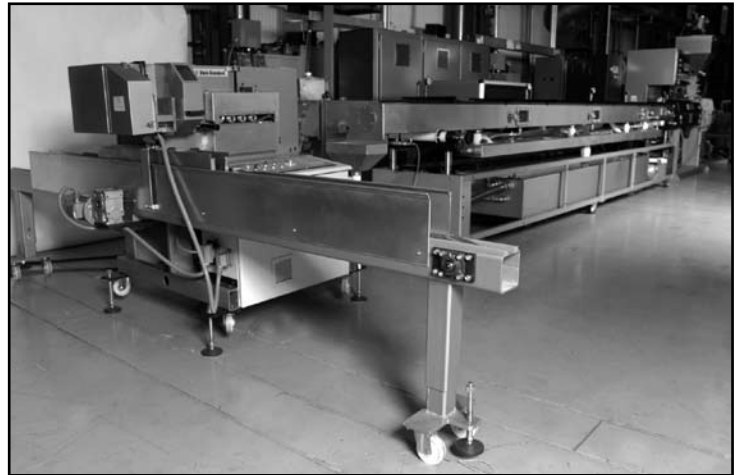
A line with an all-in-one Betopac machine for pulling, cutting and packing small serrated tubes will manufacture cotton swab sticks during the show.
