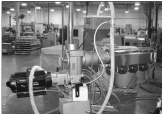
Preformed Line Products is using its new HPE extruder to manufacture air flow spoiler products for the electrical industry.
